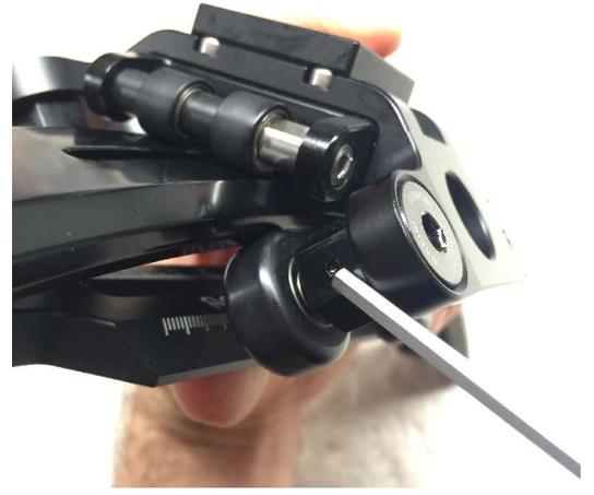
3. Each bearing shaft has a small dot, usually placed pointing forward on each axis. This is very individual to each bow though. The idea is that the dots on left and right side should be mirrored causing even pressure on both sides of the bow.
