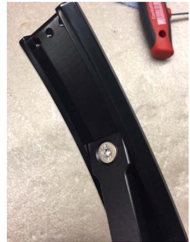
8. Be sure to check the flat heads under each bow so they are tight. If not add some loctite and tighten them again. These are also getting tremendous amount of vibration.
