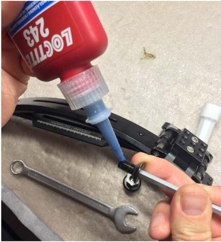
6. You can add some medium/mild loctite on the M8 thread, to hinder the shaft from moving in the future.
