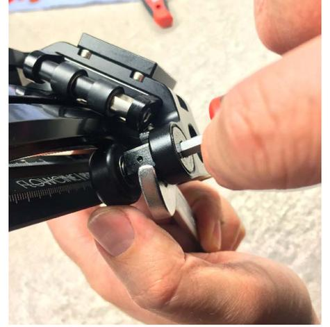
5. After finding the bearing that is too loose (rotating freely without and contact to the bow), take the wrench, and loosen the M8 flat head flowcine screw a little until you can move the shaft.
