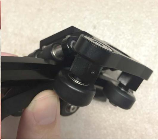
4. Generally, a dot that points inward to centre (left image) will be too loose, and a dot pointing outwards (right image) is too tight. This is highly individual to each bow though. But rotating the dot on the hexagon shaft inwards brings the bearing closer to the bow, and vice versa.
