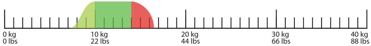
Vibration mount #02 Range 10-14kg payload (22-31lbs)
