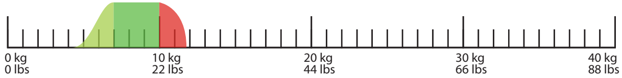
Vibration mount #01 Range 7-10kg payload (15-22lbs)
