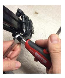
7. Or you can just directly move the hexagon shaft after loosening the M8 screw a little, and then tightening it back again. All screws are loctited at assembly, but there is a lot of vibration in each bearing assembly. Secure the M8 tightly!
