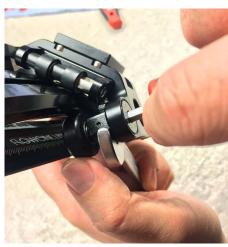
5. After finding the bearing that is too loose (rotating freely without and contact to the bow), take the wrench, and loosen the M8 flat head flowcine screw a little until you can move the shaft.
