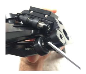
3. Each bearing shaft has a small dot, usually placed pointing forward on each axis. This is very individual to each bow though. The idea is that the dots on left and right side should be mirrored causing even pressure on both sides of the bow.
