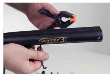
2. Remove the front cup by unscrewing the to screws with a Allen tool. Standard arms might not have these two screws, instead use a knife or other sharp object to prye the front cup from the Easyrig arm.
