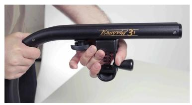
3. Pull out the cord until you can wire it around the Easyrig arm a couple of times, and then use a clamp to secure it, so the string doesnt want to go back into the Easyrig.
