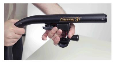
4. Loosen the plastic cup from the hook, and remove the tape that covers the knot. Untie or cut off the knot, and remove the hook and the cup from the string. We wont need the original Easyrig cord anymore.
