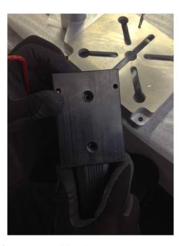
12. Finish off with a 12mm (0.47") diameter drill in the outer guides. Remember to take it slowly and remove plastic spill from the guide, and gradually go downwards when using the final 12mm size.
