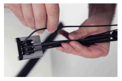
17. Take out the cord from underneath the slider, so it goes under the pulley. And then attach the slider with the knob from above. The same is true for standard arm users. First pull the string out on the bottom, then attach the pulley back into the  $\,$ Easyrig, and secure it with the two screws simultaniously.
