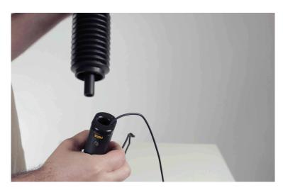
7. Unscrew and slide of the slider from the arm.
