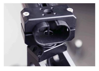
23. Tighten the two M5 screws properly, to secure that the Serene is properly fastened. No need to overdo it though! The Easyrig arm is relatively thin, and can get deformed if you go into "extreme hulk mode".
