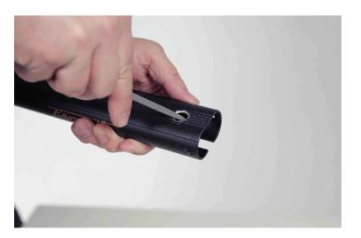
15. Now replace the cord, with the provided longer one. Be sure to follow Easyrig tutorial how to re-string the cord at: http://vimeo.com/83685316 NOTE! You must match the absorber strength in the same way you would do without the Serene, matching camera setup weight!
