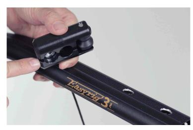
18. Open up the two brackets on the Serene arm, by unscrewing the two M5 screws at the bottom. Push the cord through the upper front hole of the Easyrig arm, and into the hole on the upper of the two brackets, so it comes out on the other side.
