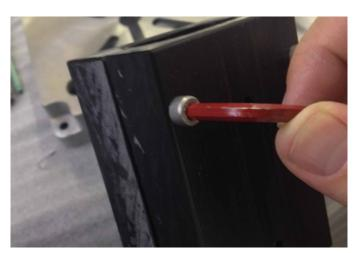
9. Insert the two M5 screws, and use a Allen tool to tighten it. Very important is to make sure the two M5 holes are facing the front of the Easyrig arm!
