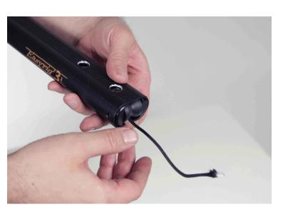
19. While pulling the string a little against you, secure the two M5 screws on the bottom. Make sure the brackets are exactly behind the two screw holes at the front!
