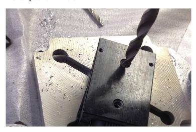
13. In order to clear the hole from any unwanted sharp aluminium bits, you can use a thin piece of cloth over the hole, and drill it again with the 12mm diameter drill. This will sand down the now exposed aluminium edges, and make the hole smoother.
