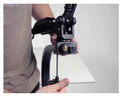
25. Remove the small m3 secure screw in the fonr, and pull the hook over the pulley to the underside of the spring arm. The cord should pull the hook against the underside. If everything feels correct and you can feel the tension from the absorber, you can now cut away extra cord if its too much to fit inside the plastic cap and seal the end with a lighter.
