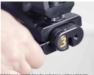
24. Pull the cord around the first pulley, on the Serene, and then pull it hard to extend it at its maximum. Put back the Easyrig hook, right before the second orange pulley, and tie the knot there. The knot should be about aligned with the front pulley after tightened.
