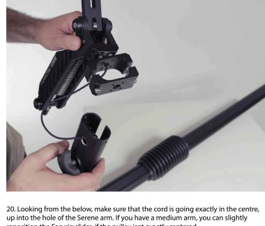
reposition the Easyrig slider, if the pulley isnt exactly centered.
