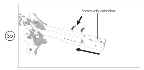
If you think the camera is too far away from your body, or if you camera setup is closer to 20kg, the innermost position is needed. You can of course choose any of the positions between fig 3a or 3b. The innermost position together with the Serene heavy extension spring gives a max weight of 195kg. Again using a smaller spring always gives a slight better performance, so when its possible downgrade to a Serene heavy or Light spring.
