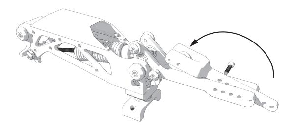
If you find the Serene arm difficult to storage. Please remove one of the supplied M5 screws, so the arm can swivel around the second one. Always release the tension of the spring before this is being done however to avoid any damages!
