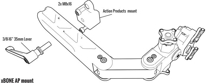
The xBONE includes a Action Products mount. Simply lock the mount on the vest with the two supplied M8x16 screws, and then insert the 3/8" Lever and lock it.
