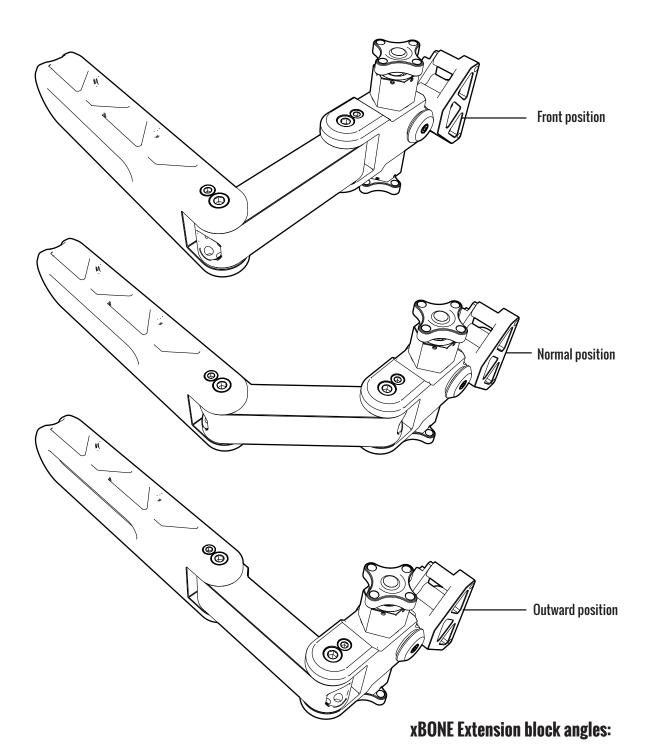
The xBONE have three different angles it can be positioned in. Each operator have to try out which angle is preferred. Each angle is in 45 degree steps, and enables the socket block to move from a front position, to a normal operation position (default) to a outward position. The different angles, combined with the three different extension blocks and a slidable Back bone gives a wide arrange of different socket block placements.
